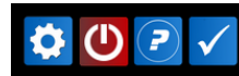
FIGURE 9 – RE-INIT BUTTON INDICATES THAT DEVICE WILL BE RE-INITIALIZED WHEN USER WILL PRESS OK BUTTON.
